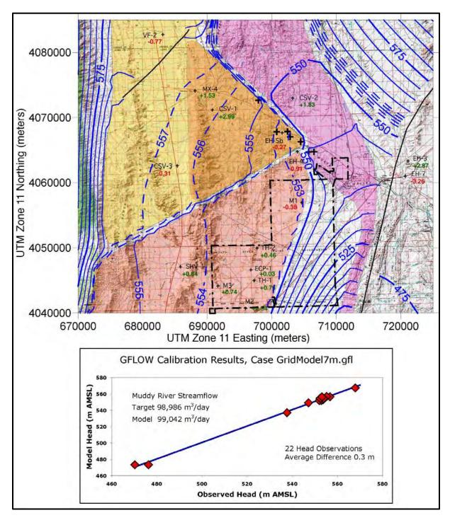
Contour interval 1 meter where dashed, 5 meters elsewhere. Bold symbols (+) show model locations of groundwater extraction by Nevada Power Company (Nevada Energy) and Moapa Valley Water District
